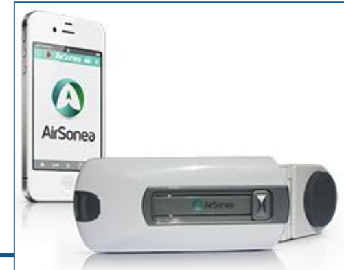
The AirSonea device, which connects to an asthma patient's smartphone and communicates with wheeze analysis algorithms on iSonea's server.
